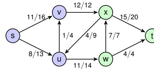
$$\begin{aligned} S &= \{s, u, v\} \\ T &= \{x, w, t\} \\ c(S, T) &= 26 \\ f(S, T) &= 19 \end{aligned}$$
